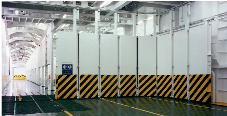
Figure 25: Top stowing Jalousie flood control door [55]
